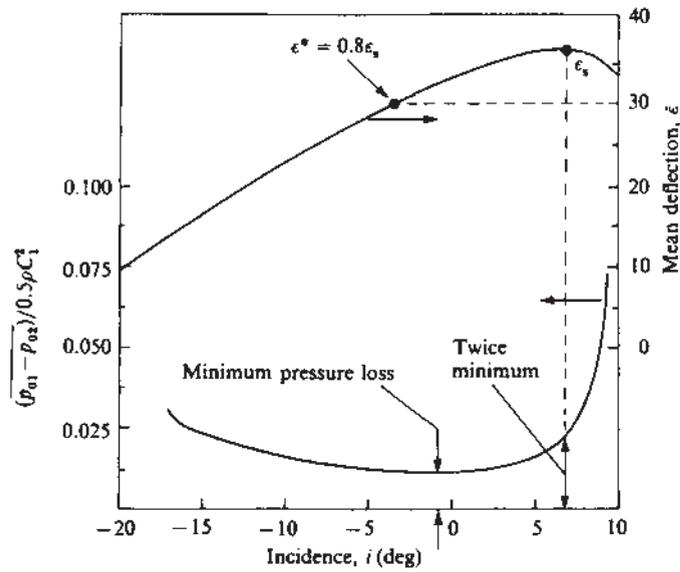
**Figure 5.9** Cascade mean deflection and pressure loss curves.
