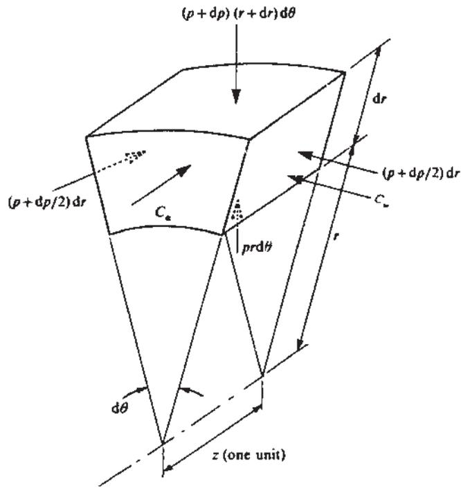
**Figure 5.11** Pressure forces on a fluid element.
