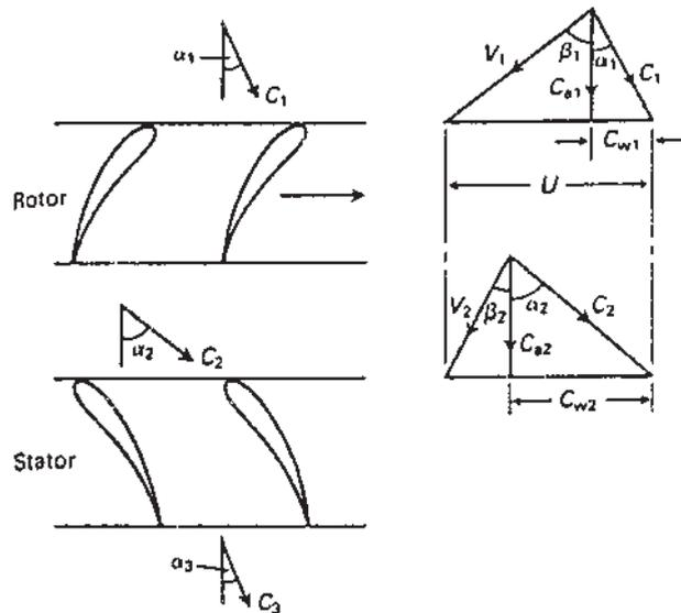
**Figure 5.4** Velocity diagrams for a compressor stage.
