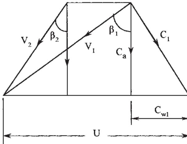
**Figure 5.14** Velocity triangle at the mean radius.
