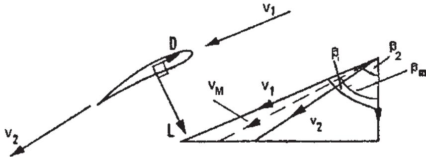
**Figure 5.6** Lift-and-drag forces on a compressor rotor blade.
