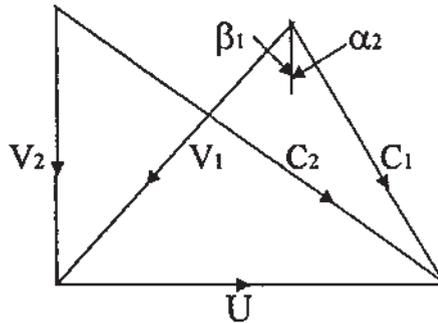
**Figure 5.17** Combined velocity triangles for Example 5.6.
