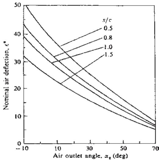
**Figure 5.20** Cascade nominal deflection versus air outlet angle.
