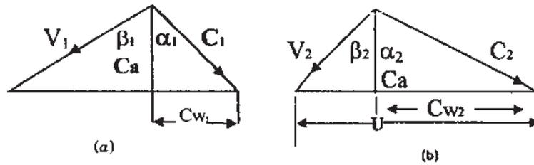
**Figure 5.18** Velocity triangles (a) inlet, (b) outlet.
