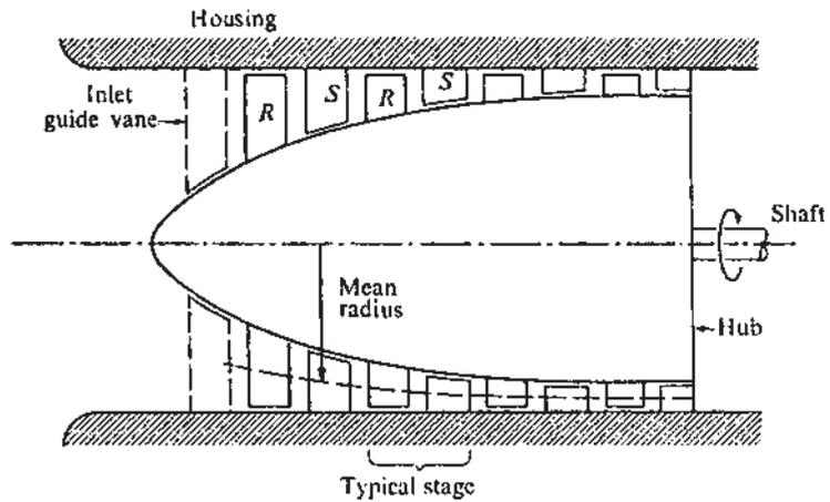
**Figure 5.3** Schematic of an axial compressor section.
